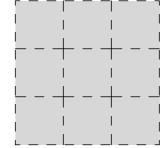
2' X 2' TIN CEILING TILE TO BE REMOVED AND SALVAGED FOR REUSE
